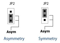
The default factory setting of FBs-CM5H is Terminator - CH1~CH4 all installed Working mode - Symmetry
